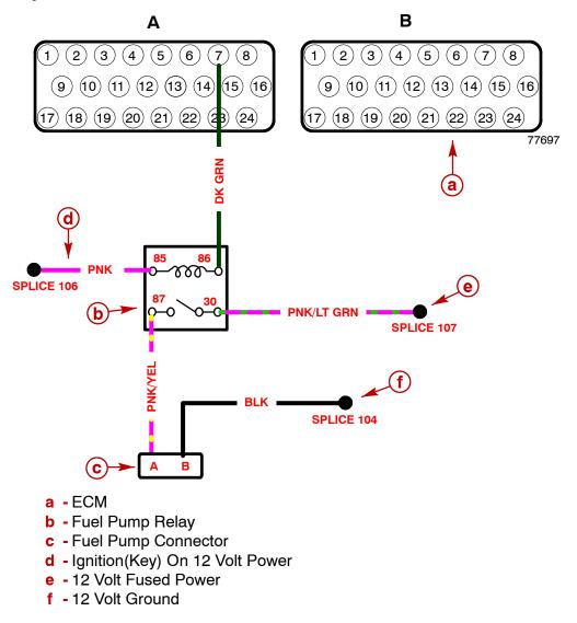
Upon key ON, the fuel pump relay receives 12 v battery power through the fuses at terminal 30. The relay powers both fuel pumps and signals the ECM that the engine is ready to start. Listen at key ON for both fuel pumps to operate.
