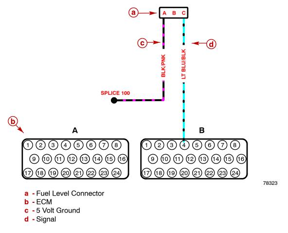
The fuel level sensor circuit supplies the ECM with the fuel level. It is located on the port rear of the engine.
