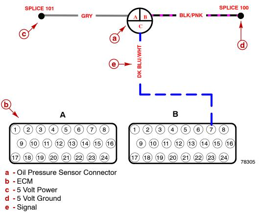
The oil pressure sensor measures oil flow through the oil galleries. It is located on the rear port side of the engine.
