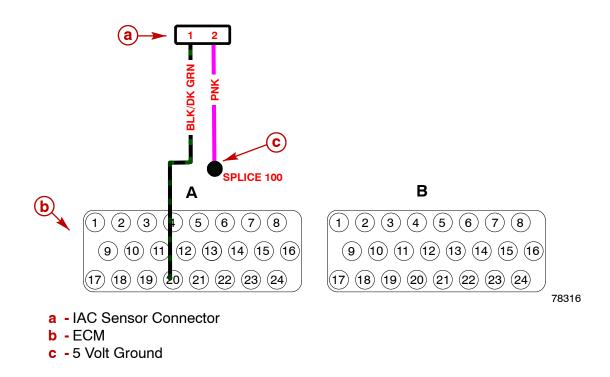
The idle air control (IAC) value is a 12 volt circuit powered by the MPR. It is located at the top rear of the engine.
