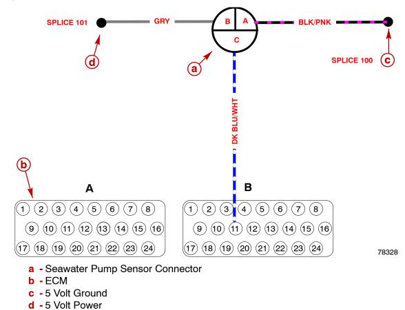
The seawater pump sensor measures water inlet pressure or water block pressure. It is located at the seawater pump inlet hose. Normal pressure ranges are 7-34 kPa (1-5 psi) at idle and 48-117 kPa (7-17 psi) at WOT. To check if sensor is within range, the diagnostic tool reading with key ON should be approximately 0.
