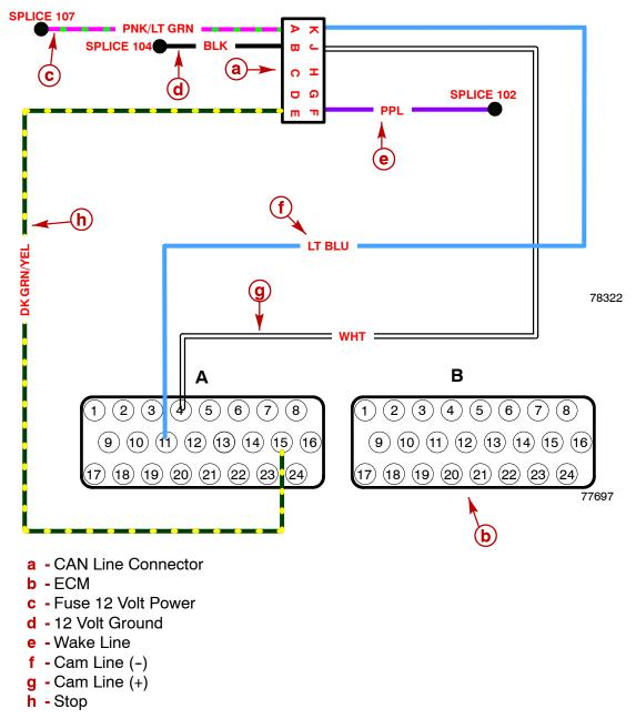
The CAN circuit powers the Smartcraft gauges on mechanical throttle and shift engines. It is located on the rear of the engine on the upper port side. The gauges receive power through the BUS power and ground. Gauge information (RPM, TEMP, TRIM) is sent through the CAN leads.
