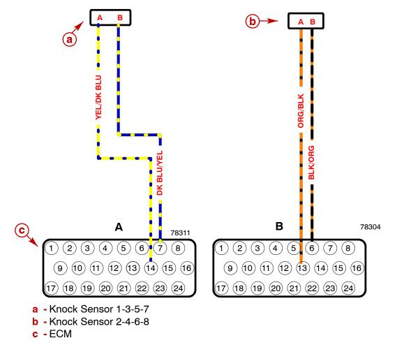
The knock sensors detect engine detonation or spark knock and send a voltage signal to the ECM. They are located on the lower half of the engine on both the port and starboard sides. As the sensor detects knock, the voltage output level increases and signals the ECM of the problem.
