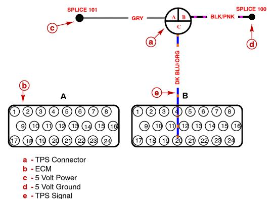
The throttle position sensor (TPS) sends throttle plate angle information to the PCM. It is located on the throttle body. Signal voltage should vary from 0.5 volts at idle to 4.7 volts at WOT. If the TPS malfunctions, the ECM will reset to a default value.
